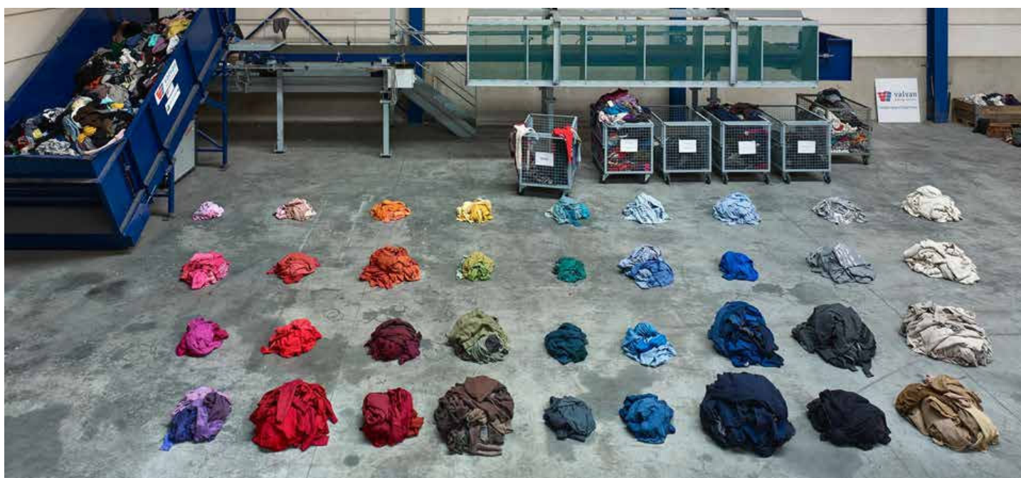
Sorting clothing for recycling with Fibersort: Automated sorting 45 categories based on colour, structure and fibre, at 900kg per hour with Near-infrared spectroscopy (NIR)
